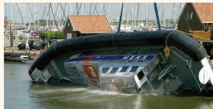
▲ Top Left and Bottom Right: Shooting from a low angle to enhance the sense of the height and roughness of the waves; Top Right: Low camera angles and heavy surf are always good for some spectacular shots; Bottom Left: Capsize test of Dutch lifeboat
